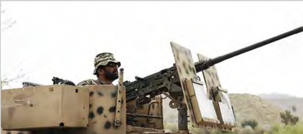
An Afghan gunner in a HMMWV outfitted with an older gunner protection kit and no Overhead Cover in 2017. (Photo provided by the Asymmetric Warfare Group)
