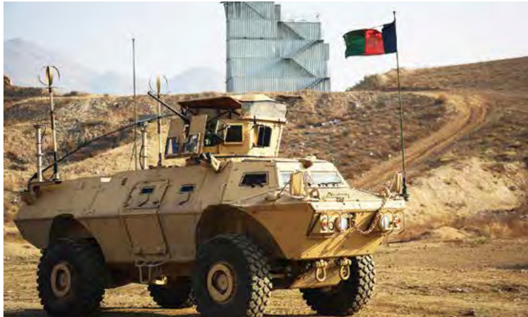
A Mobile Strike Force Vehicle provided to an Afghan commando unit. MSFVs, such as the one pictured above, provide more mobility, protection, and firepower than the ANSDF’s HMMWVs. (U.S. Army photo by Connor Mendez)
