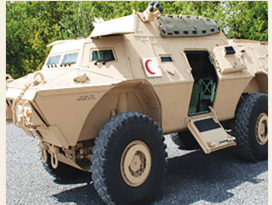
An ambulance variant of the Mobile Strike Force Vehicle. (Photo provided by the U.S. Army Program Executive Office for Combat Support & Combat Service Support)
