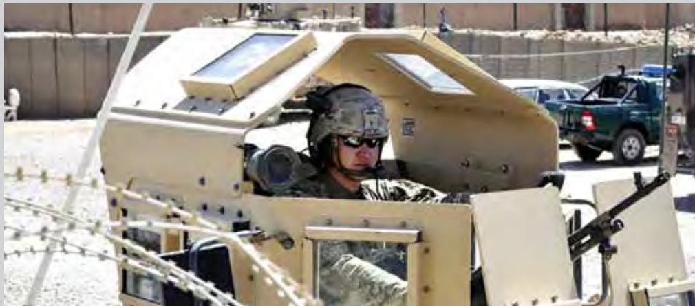
A U.S. gunner in Afghanistan in a HMMWV outfitted with the U.S. Objective Gunner Protection Kit and Overhead Cover in 2013. (Photo by Jessi McCormick)
